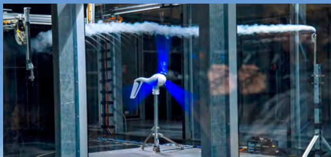
UT Dallas invested approximately $5 million to build the Boundary Layer and Subsonic Tunnel (BLAST) which opened this year. The tunnel features two test sections, the boundary layer test section (up to 76 mph with 100 feet of optical access) and the subsonic test section (up to 112 mph). Image shows visualization of air flow past a wind turbine with smoke generator inside BLAST.
