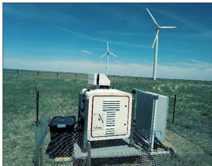
Deployment of the UTD mobile LiDAR station at a wind farm on complex terrain in Colorado
