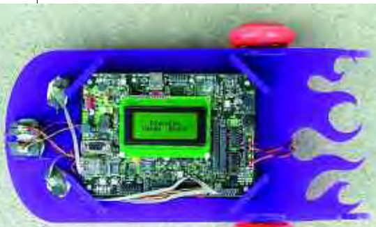
The Blackfin Handy Board was developed by Asst. Prof. Fred Martin in collaboration with Analog Devices Inc. This new version of the original, which Martin designed, is based on ADI’s Blackfin Processor.
