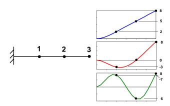
Fig 6a – Beam 3 DOF Model
