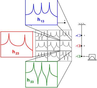
Fig 10b - Roving Response Test Scenario
