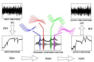
Fig 23 - Schematic Overviewing the Input-Output Structural Response Problem
