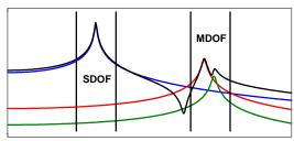
Fig 21 - Curvefitting Different Bands using Different Methods
