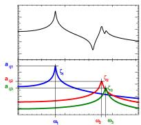
Fig 20 - Breakdown of a Frequency Response Function
