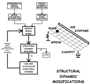
Fig 29 – Schematic of the SDM Process
