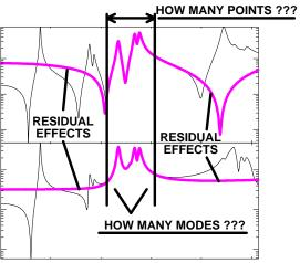
Fig 22 - Curvefitting a Typical FRF
