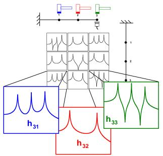
Fig 10a - Roving Impact Test Scenario
