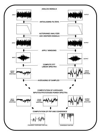
Fig 11 - Anatomy of an FFT Analyzer
