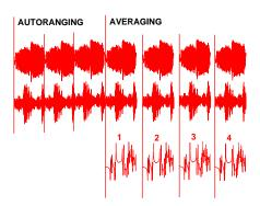
Fig 16 - Sine Chirp Excitation Without a Window
