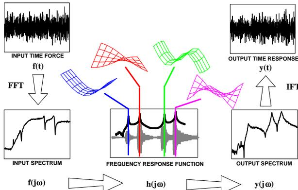
Fig 23 - Schematic Overviewing the Input-Output Structural Response Problem
