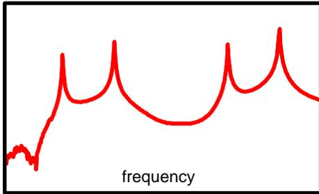
Fig 3 - Simple Plate Frequency Response Function
