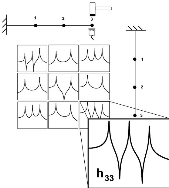
Fig 7a – Drive Point FRF for Reference 3
