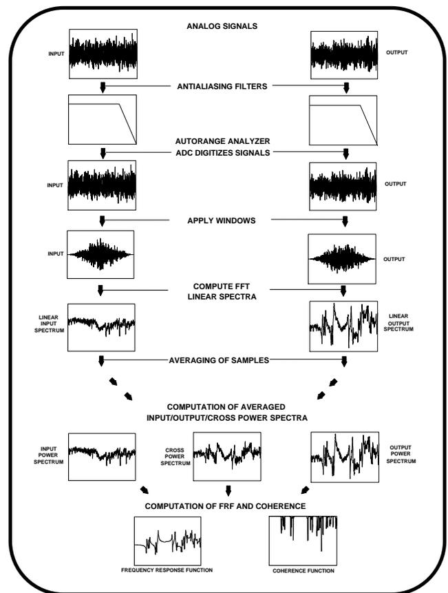
Fig 11 - Anatomy of an FFT Analyzer
