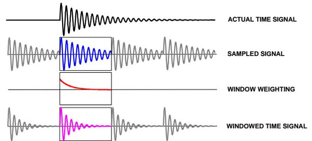
Fig 13 - Exponential Window to Minimize Leakage Effects
