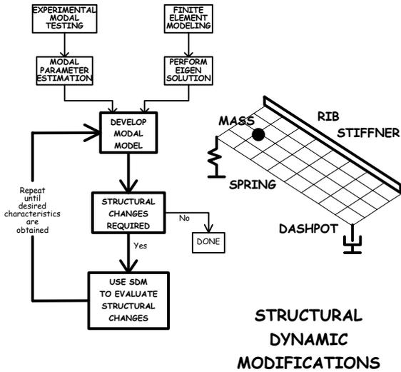
Fig 29 – Schematic of the SDM Process
