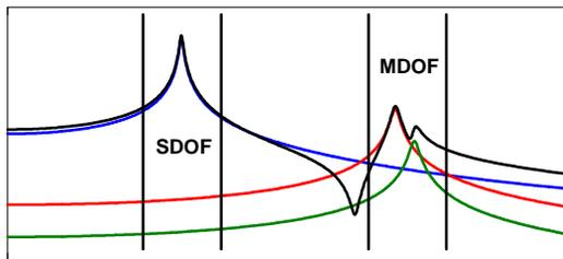
Fig 21 - Curvefitting Different Bands using Different Methods
