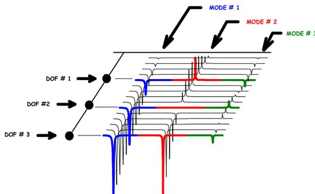
Fig 9 - Waterfall Plot of Beam Frequency Response Functions
