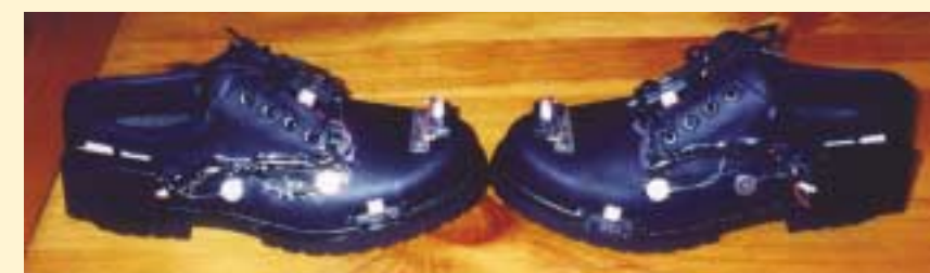
Vibrating motors connected to sensors on the shoes of blind wearers identify obstacles in their vicinity. The system is controlled by a pack containing three AAA batteries and all the circuitry.
