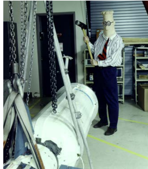
Figure 3a: Impact test on missile hung at locations that are close to the nodes of the first bending modes
