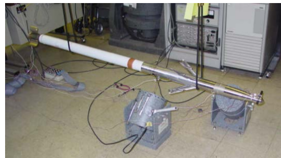
Figure 3b: Shaker test on missile hung at locations that are close to the nodes of the first bending modes
