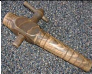
A barrel spigot , made of wood and cork, used in wooden barrels that store wine.
