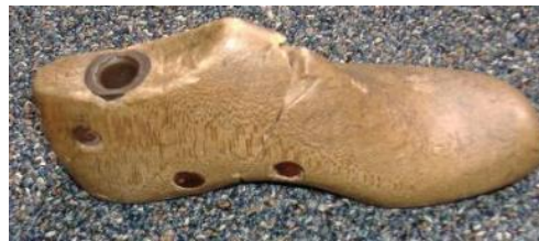
A shoe form is a tool for making handmade leather shoes. There is a form for each shoe size.
