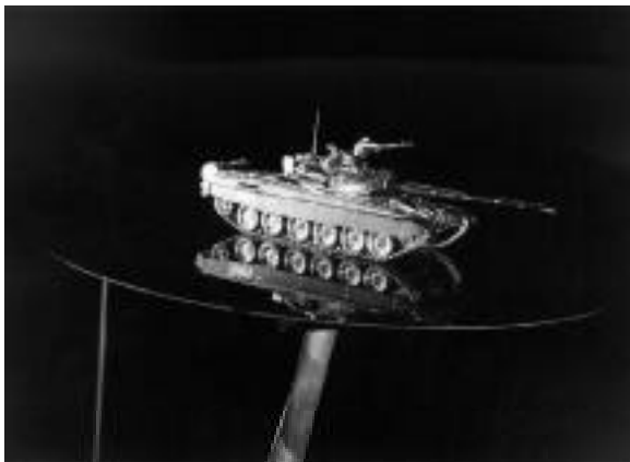
Figure 7. View of the scale-model tank shown mounted on a smooth groundplane
