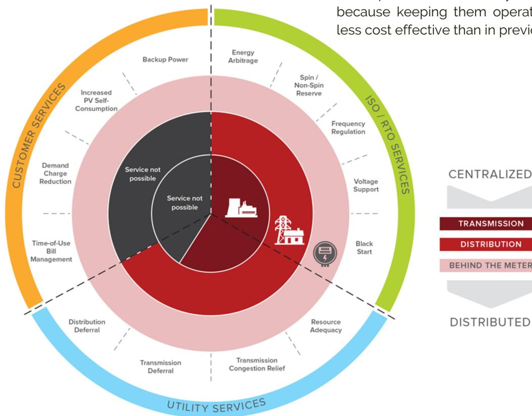
Fig. 9. Grid energy storage can provide up to 13 services three stakeholder groups, including utilities, independent system operators (ISOs) and regional transmission organizations (RTOs), and customers. Retrieved from The Economics of Battery Energy Storage Report by Rocky Mountain Institute: <https://rmi.org/insight/economics-battery-energy-storage/>
