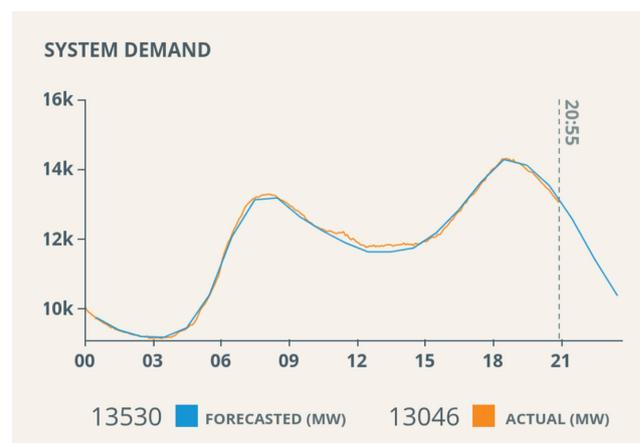
Fig. 2. System demand real time data retrieved on October 23, 2019 for forecasted system demand (blue) and actual system demand (orange). Retrieved from [www.iso-ne.com](http://www.iso-ne.com)
