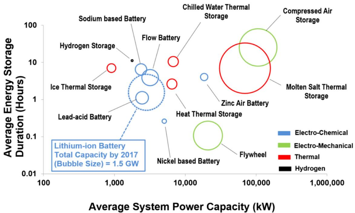
Fig. 5. Average characteristics of energy storage systems built worldwide between 1958 and 2017. Retrieved from <https://www.nrel.gov/docs/fy19osti/71714.pdf>
