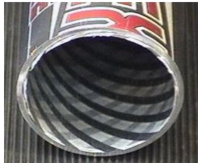
Fig. 2 Cut hollow aluminum bat
