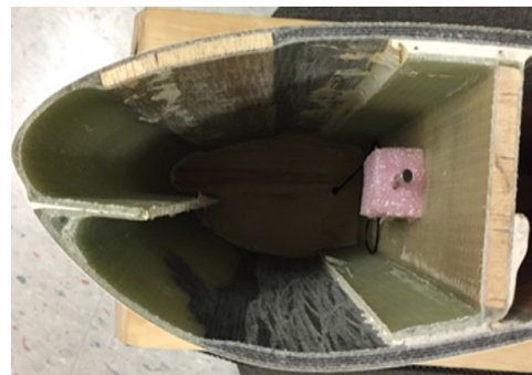
A close-up of a blade-internal microphone used for in-lab acoustic detection tests.
