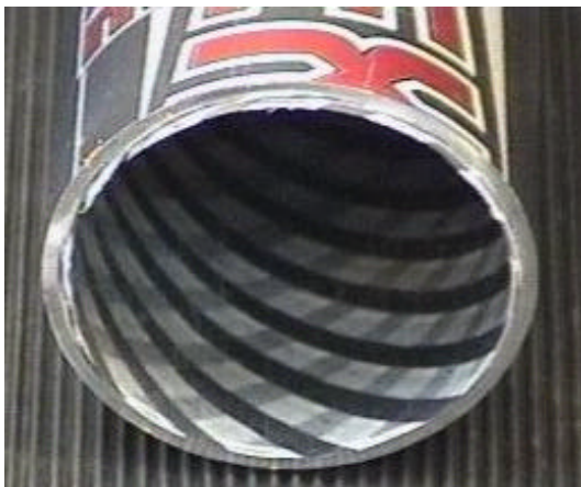
Figure 2 - Cross section of aluminum bat.
