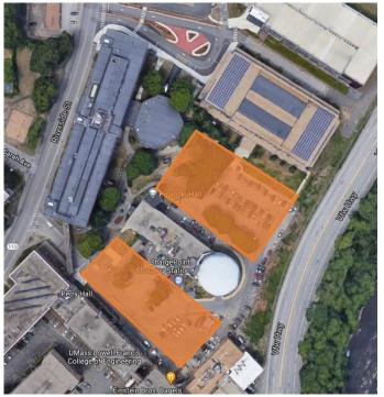
Good Option B1 and B2 geothermal borefield
