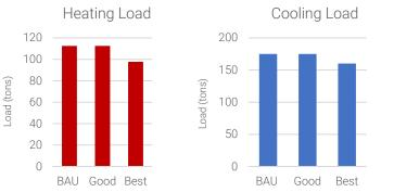
ECM 6a - Air-side Energy Recovery - 70% (Single Wheel) ECM 7b - Water-side Systems - Standalone AWHP ECM 9a - Plumbing - Low Flow Fixtures
