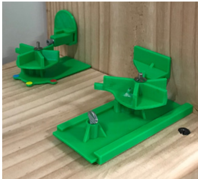
Printed Prototypes for Two Designs of the Wind Turbine Foundation Monitoring Sensor.
