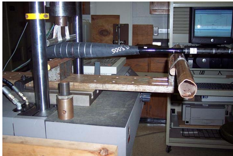
Figure 5 Barrel compression test setup
