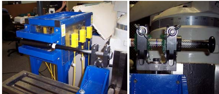
Figure 14 Grip fixture on air cannon
