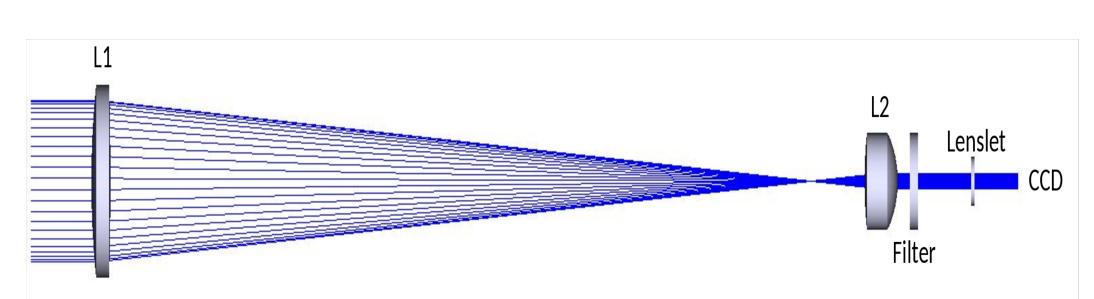
**Above:** Implementation of the PICTURE-C low-order wavefront sensor. Light reflected off the IWC is compressed and fed into the SH which measures spot displacements relative to a reference wavefront.
