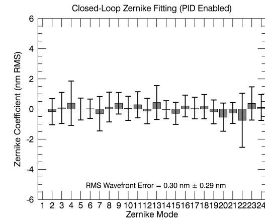
**Above Left:** Spotfield pixel deviations while the PID controller is enabled. **Above Right:** Zernike modes corresponding to the corrected wavefront.
