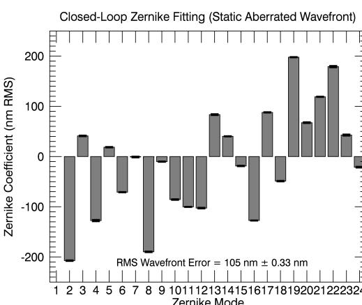
**Above Left:** Step response of the SH sensor. **Above Right:** Zernike modes corresponding to the aberrated wavefront.
