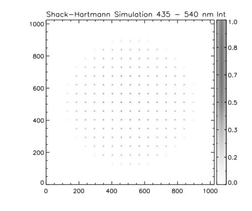
**Above Left:** Independent dynamic range of Zernike modes for the PICTURE-C SH sensor. **Above Right:** A simulated image of the PICTURE-C spotfield pattern produced by the SH sensor. 154 spots are used to measure the wavefront.
