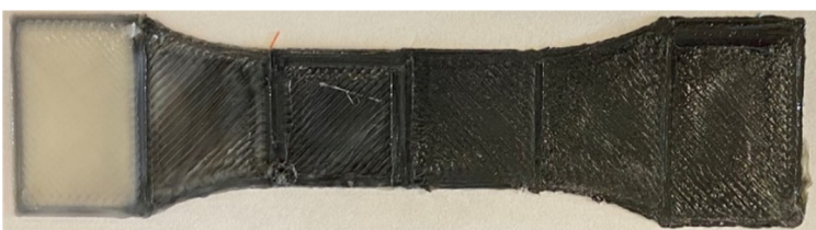
Figure 3. (left) Graduated tensile bar, and (right) Flexible hinge with TPU transitioning to PLA
