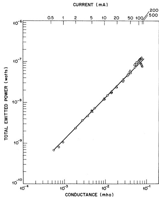
FIG. 2. Dependence of total radiated power on conductance of impact-ionized GaAs sample at 4.2°K. Current pulses 200 (open circles) and 20  $\mu$ sec (open triangles) long were applied at a repetition rate of 1.5 kHz.
