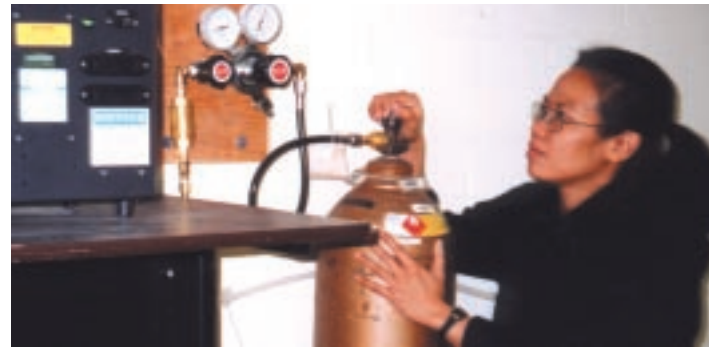
Panhathai Buasri, a doctoral candidate in electrical engineering, opens a hydrogen tank valve that allows the gas to flow into fuel cells, where it will combine with oxygen to generate electricity. Prof. Ziyad Salameh says fuel cells are a "clean, noiseless source of energy."
