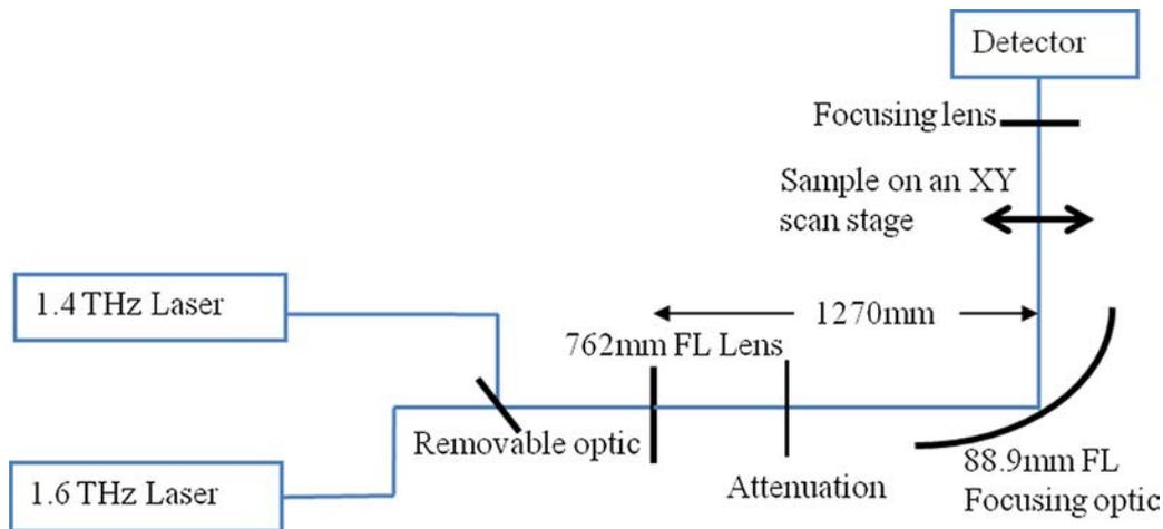
Fig. 1. Schematic of experimental layout.
