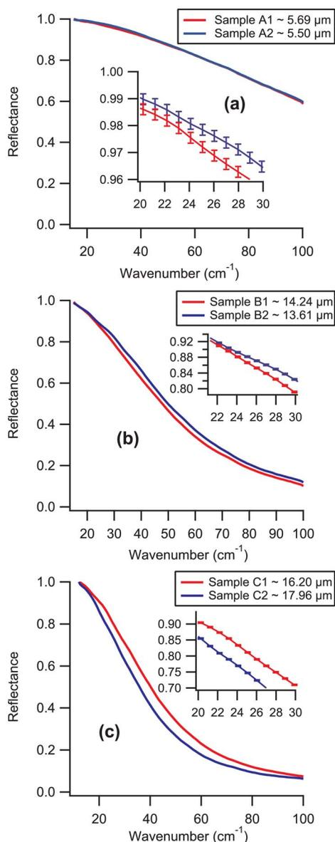
Fig. 2. (Color online) Terahertz reflection spectra of two samples differing in rms roughness by (a)  $0.19 \mu\text{m}$ , (b)  $0.63 \mu\text{m}$ , and (c)  $1.76 \mu\text{m}$ . Inset shown for wavenumbers  $20 \text{ cm}^{-1}$  to  $30 \text{ cm}^{-1}$  with error bars.
