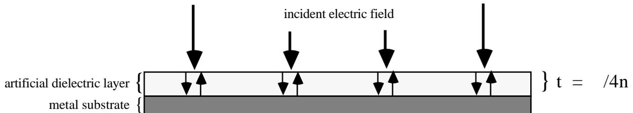
Figure 1. The FIRAM depicted is a resonant absorption structure which consists of a quarter wavelength thick homogeneous lossy dielectric surface on a metal plate.
