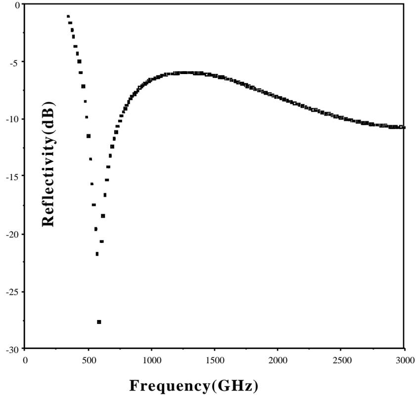
Figure 2. The reflectivity as a function of frequency for an artificial dielectric material specifically matched in metal loading and thickness to provide an RCS reduction of  $-27\text{dB}$  at 0.585 terahertz.
