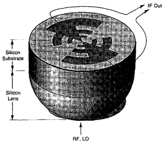
Fig. 2. Log-periodic toothed antenna fabricated on an extended hemispherical silicon lens (1.3 mm in diameter).
