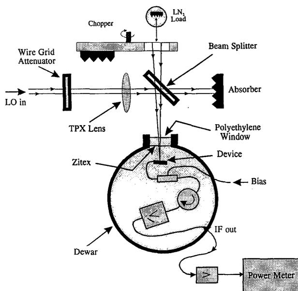
Fig. 4. Optical layout for noise measurements.
