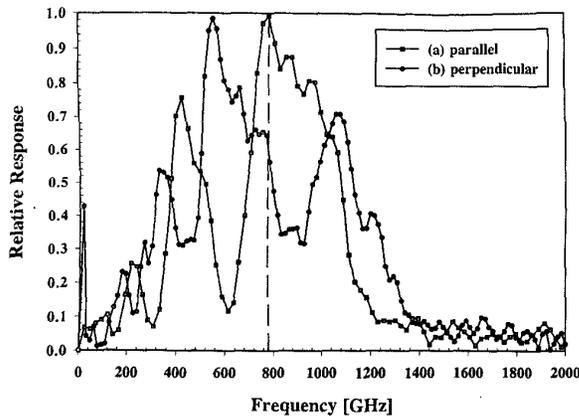
Fig. 5. FTS spectra of the device of Antenna A for (a) device orientation parallel to the FTS polarization, and (b) perpendicular to the FTS polarization.
