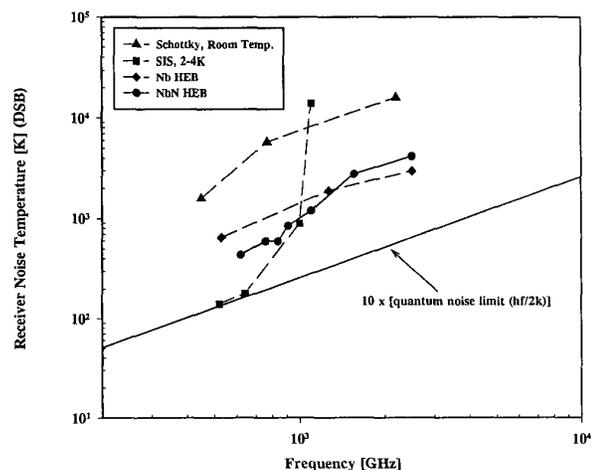
Fig. 1. Receiver noise temperature for receivers in the THz frequency range.
