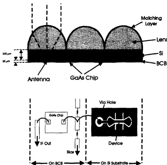
FIG. 4. A portion of an HEB terahertz focal plane receiver array.
