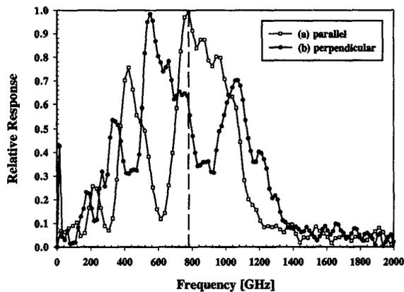
FIG. 3. FTS spectra of the device with the larger antenna for (a) device orientation parallel to the FTS polarization, and (b) perpendicular to the FTS polarization.
