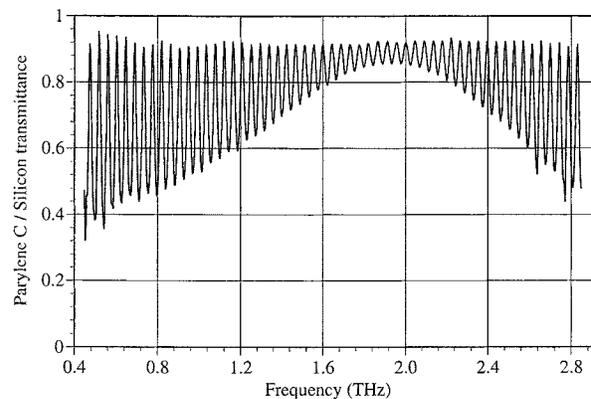
Fig. 2. Terahertz transmittance of a high-resistivity ( $\rho > 20\,000\ \Omega\text{-cm}$ )  $1011\text{-}\mu\text{m}$  thick silicon substrate coated with  $24.0\ \mu\text{m}$  of parylene C on both sides.
