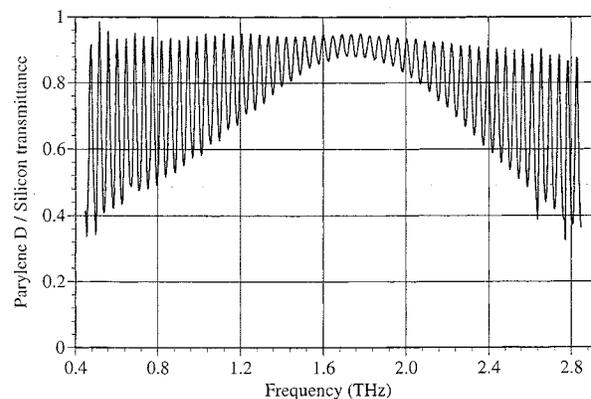
Fig. 3. Terahertz transmittance of a high-resistivity ( $\rho > 20\,000\ \Omega\text{-cm}$ )  $1011\text{-}\mu\text{m}$  thick silicon substrate coated with  $26.5\ \mu\text{m}$  of parylene D on both sides.
