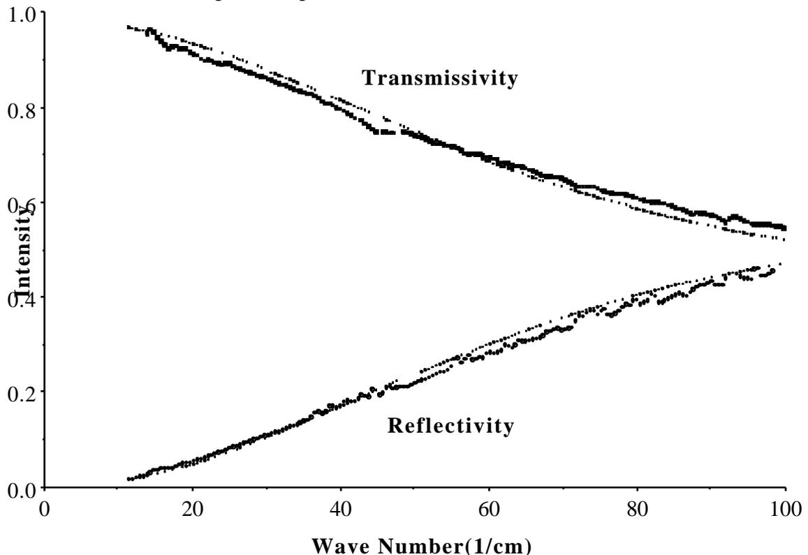
**Figure 4.** The measured transmissivity and reflectivity as a function of frequency ( $1/\text{cm}^{-1}$ ) is shown for the  $7 \mu\text{m}$  thick diamond film, sample "b", and compared to the model.
