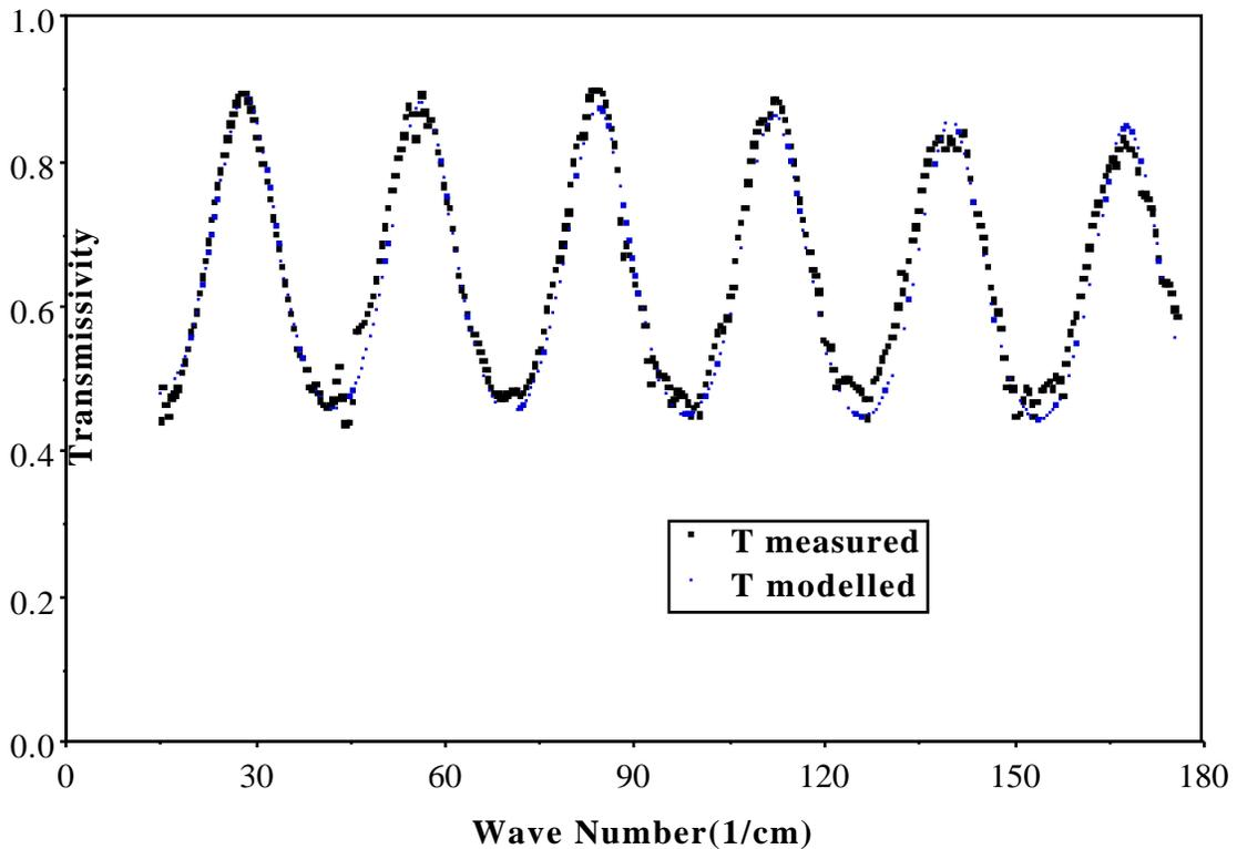
**Figure 3.** The measured transmissivity as a function of frequency ( $1/\text{cm}^{-1}$ ) is shown for the  $72\mu\text{m}$  thick diamond film, sample "a", and compared to the model.
