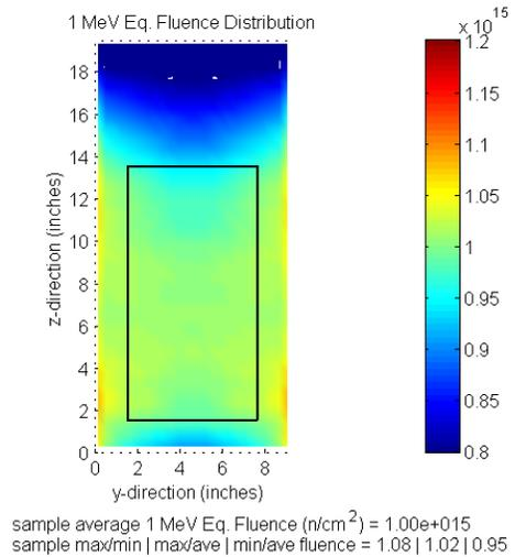
**Above Left:** Depicts the calculated 1 MeV equivalent neutron fluence distribution from side to side of the sample holder (i.e., view from above the sample holder, where the x-direction is along the side of the reactor core, y-direction is distance from the reactor core).
