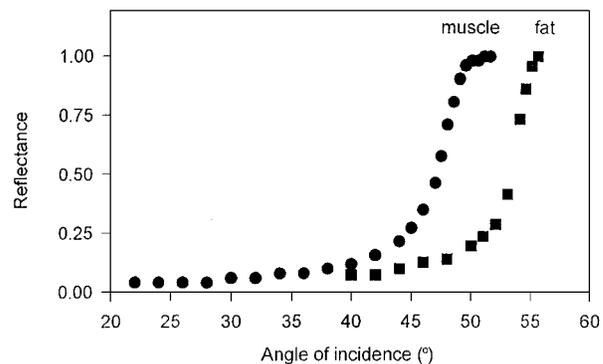
Fig. 3. Reflectance of 2.09- $\mu\text{m}$  laser radiation at the (squares) sapphire-muscle fat and (circles) sapphire-water interfaces.
