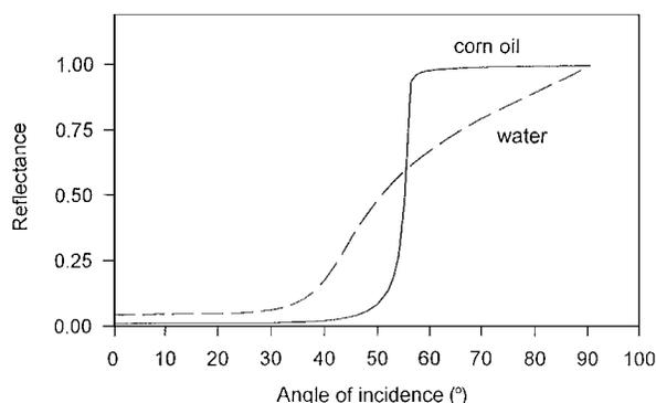
Fig. 4. Calculated reflectance of 2.79- $\mu\text{m}$  laser radiation at the sapphire-corn oil and sapphire-water interfaces.
