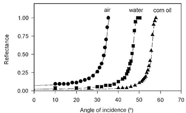
Fig. 2. Reflectance of 2.09- $\mu\text{m}$  laser radiation at (triangles) the sapphire-corn oil, (squares) sapphire-water, and (circles) sapphire-air interfaces. The curves show the theoretical predictions obtained with Eq. (1) and the values in Table 1.
