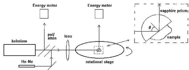
Fig. 1. Experimental setup: pol/atten, polarizer-attenuator.
