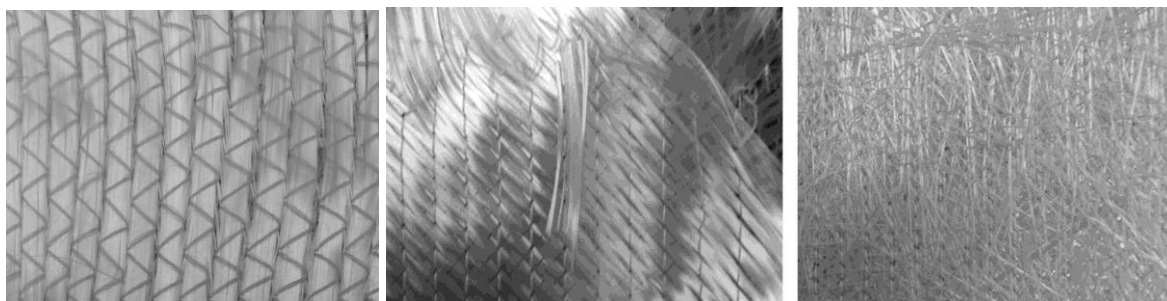
Figure 2.1.1 Examples of non-crimp, double bias non-crimp, and random mat fabrics
