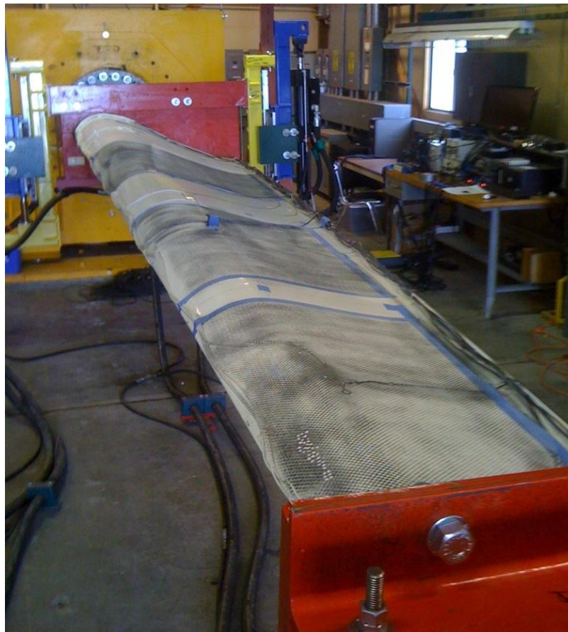
Figure 2.5.1 LANL defect-free blade test setup at NREL with DIC patterning.
