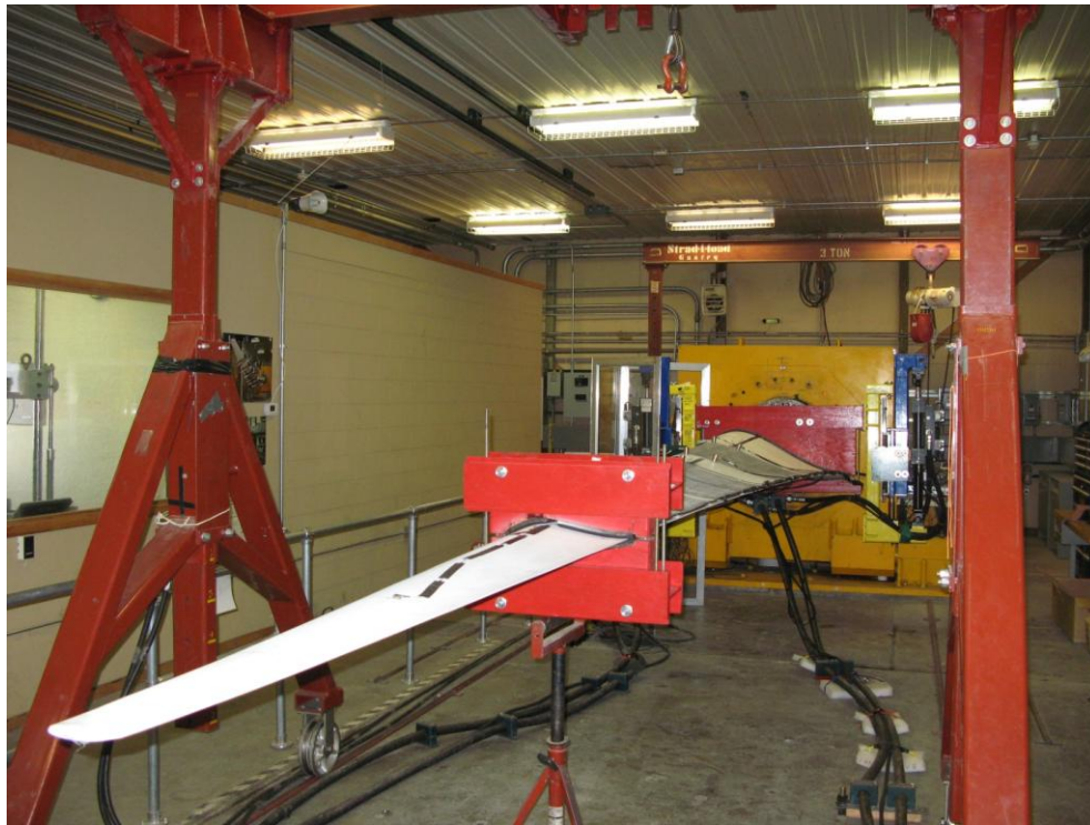
Figure 2.6.1 NREL flapwise fatigue test setup for 9-meter UMass Lowell defect blade.
