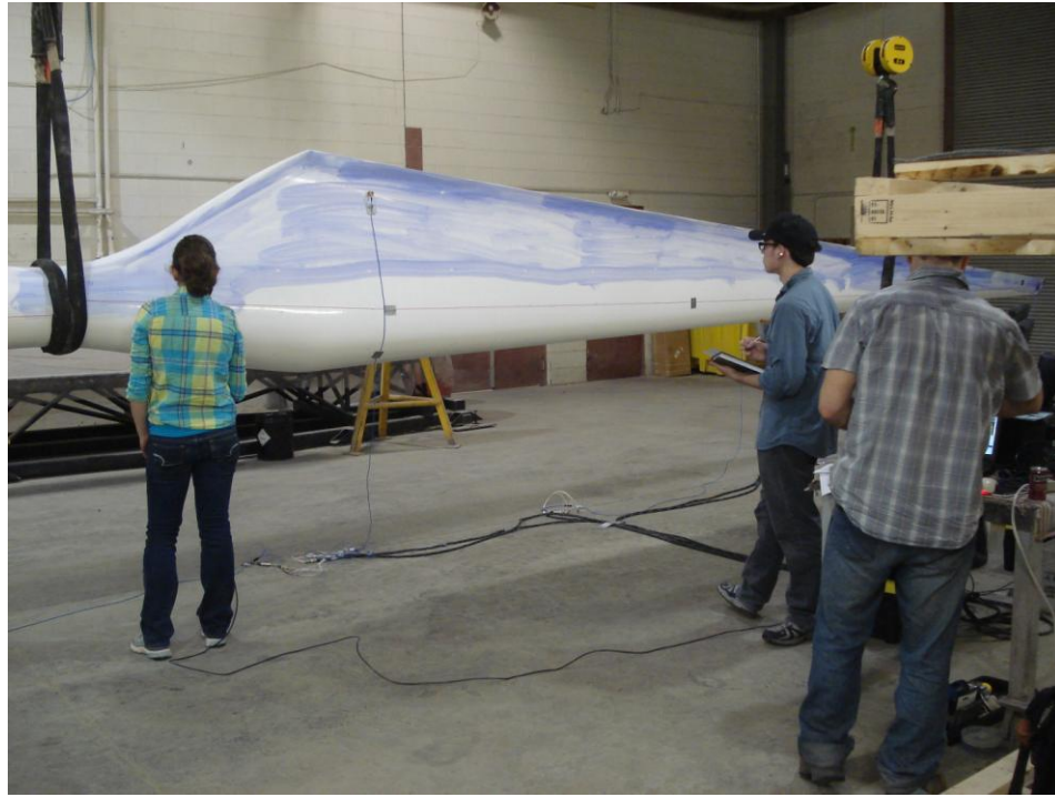
Figure 2.7.1 Free-free modal test setup for 9-m UMass Lowell defect blade at TPI.
