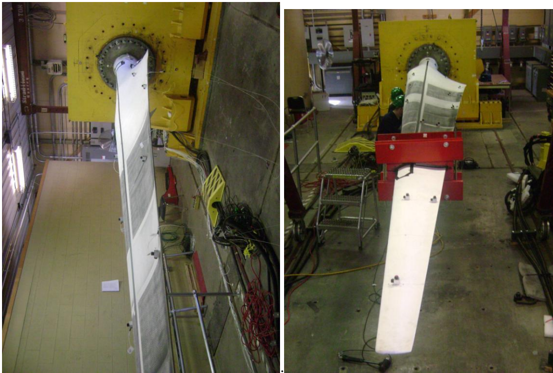
Figure 2.7.2. 9-m UMass Lowell defect blade clamped (a) without, and (b) with the saddle at NREL
