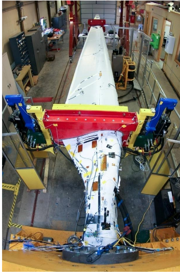
Figure 4. Fatigue test configuration of the CX-100 at the NWTC.
