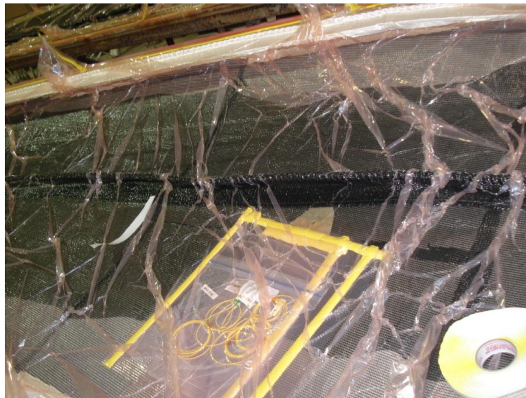
Figure 5. Fiber egress ends terminated with FC/APC connectors and double bagged during the infusion process.
