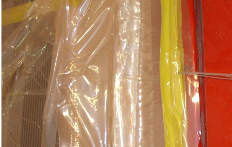
Figure 4. Optical fiber ingress through bag seam at trailing edge for vacuum and infusion.
