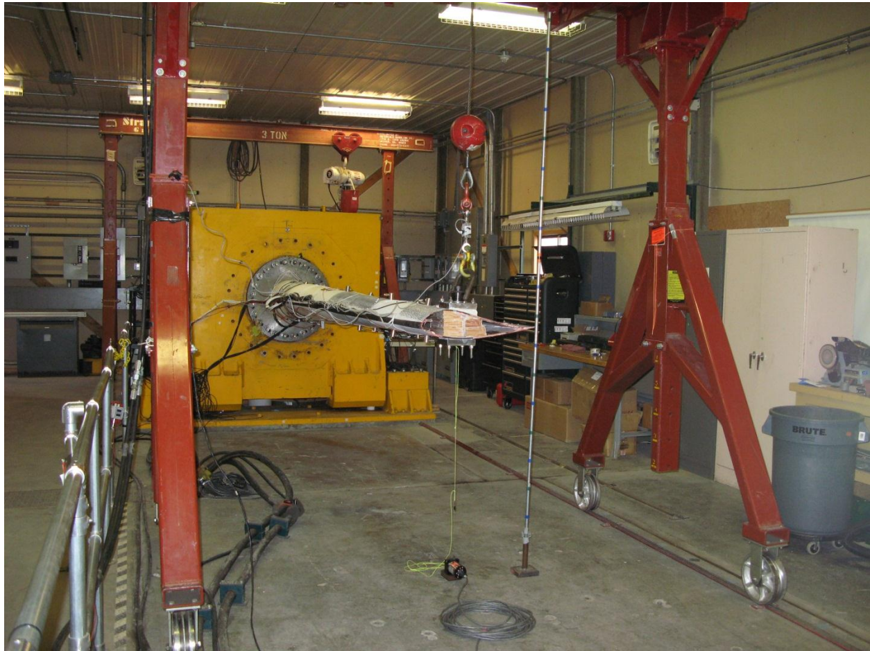
Figure 8.10 – Post Fatigue Failure Residual Strength Flapwise Static Test
