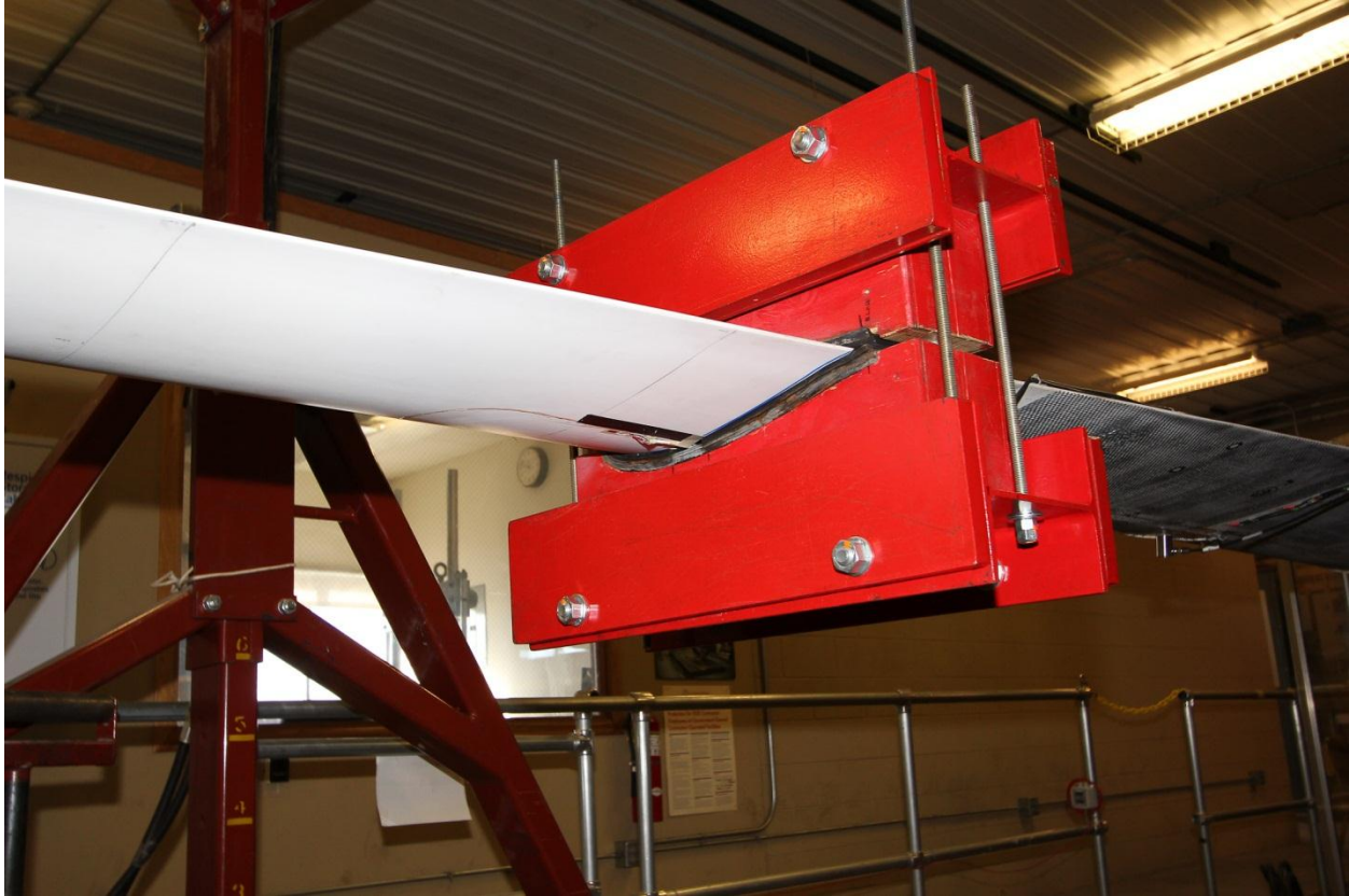
Figure 5.3 – 6.75-m Ballast Saddle
