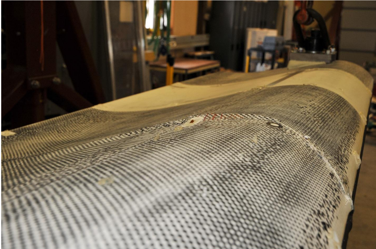
Figure 8.13 – Static Test Buckling Failure (HP Side at 3.5-m Station)
