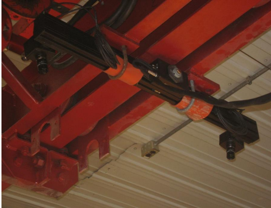
Figure E.8 Camera bar mounted to overhead gantry.
