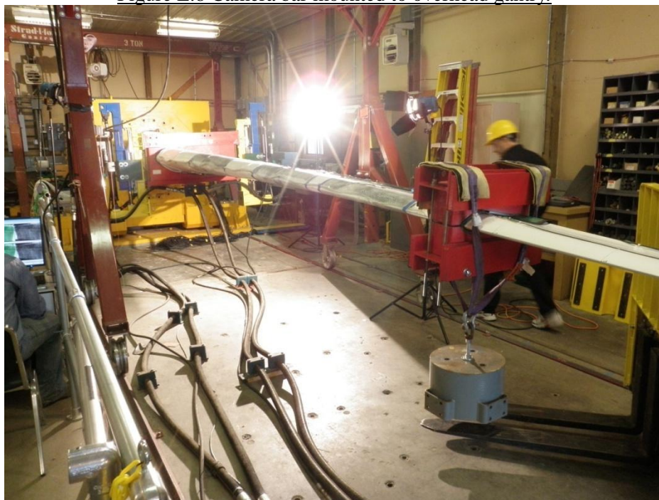
Figure E.9 LANL CX-100 nine meter blade under load.
