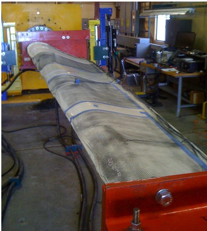
Figure E.7 LANL defect free blade with DIC patterning.
