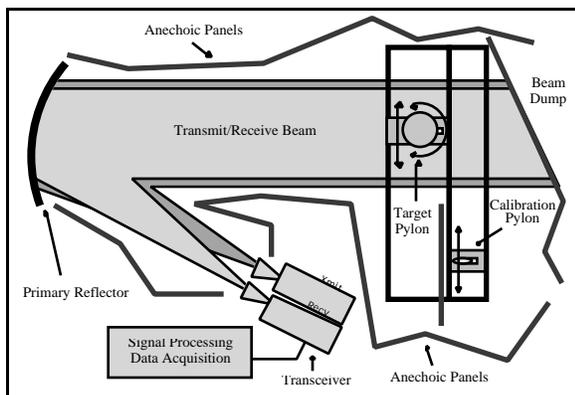
Figure 1. Top View of Compact Range.
