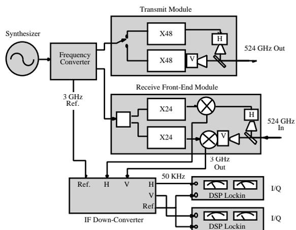
Figure 2. Block diagram of 524 GHz Transceiver
