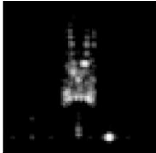
Figure 8. Incoherent sum of the 64 ISAR images measured from  $4.5^\circ$  -  $5.5^\circ$  in  $0.015^\circ$  increments.
