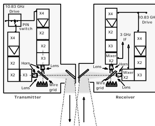
Figure 3. Diagram of 524 multiplier chain modules.
