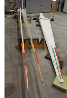
1.5MW Turbine, 10% Blade Growth Simulation Results
