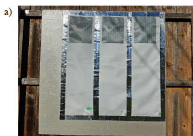
Figure 1. a) Photograph of riblet films exposed in outdoor environment in DFW area; b) Drag reduction percentage of riblet film after 3-month exposure to outdoor environments.
