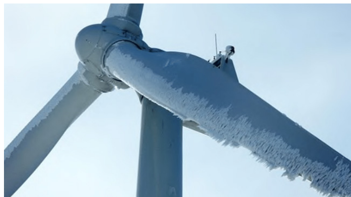
Figure 1. Example of icing on wind turbine blades.
