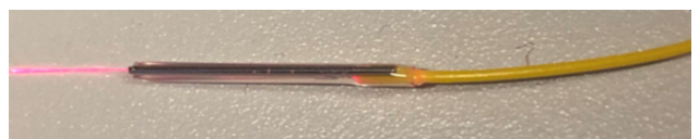
Figure 2. Fiber-optic epoxy resin cure sensor with light passing through
