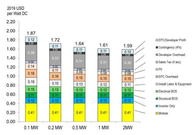
Figure 1 - NREL 2020 U.S. Benchmark: Commercial Rooftop PV System Costs (2019 USD/W-DC)
