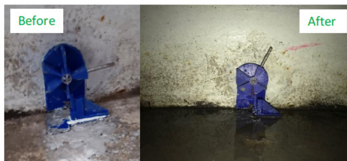
Performance of the displacement-monitoring indicator operating at the base of a wind turbine tower's harsh environment.
