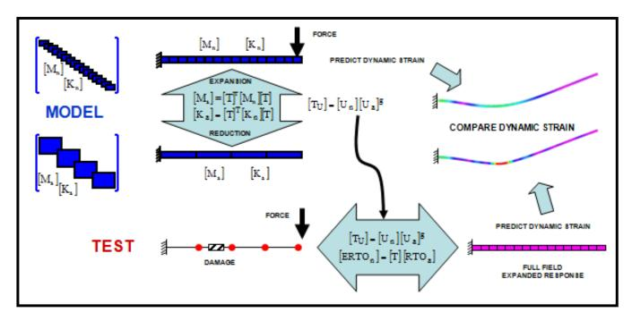
Using a limited set of measurements, the full field measured data can be compared to analytical model predictions to identify changes in load distribution which is manifested in strain difference distributions. While more work is continuing on this technique, there is great promise due to the significant wealth of data that can be obtained from full field information. Effort on data mining and manipulating the data for positive indications will be the focus of future work.
