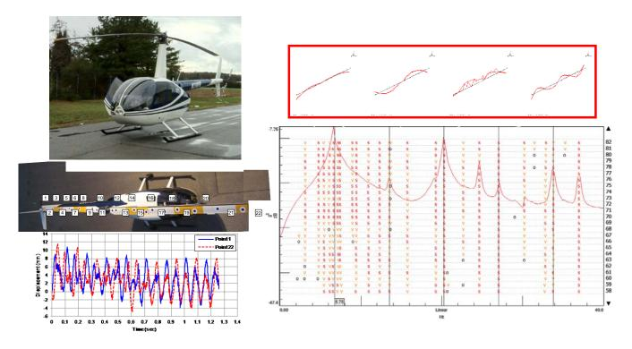
Dynamic measurements were made on a Robinson 44 helicopter rotor blades using dynamic photogrammetric techniques while in operation and in hover. The data was acquired and processed using operational modal analysis (output only data) techniques using LMS Test.LAB and operating modes were obtained.
