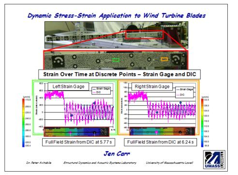
Often times, wind turbine blades are subjected to static and dynamic testing to identify the performance levels that can be achieved for a particular configuration. Many times only a handful of strain gages are deployed to capture that information.
