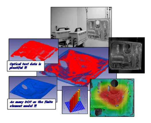
Digital image correlation has been mainly used for static applications. In the current research, DIC is used to identify structural dynamic characteristics. Normal mode testing is employed to obtain characteristic mode shapes for comparison to the finite element model. The DIC provides tremendous resolution which has been the stumbling block for most traditional approaches employed.
