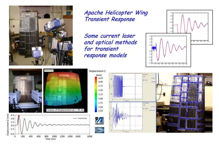
Evaluation of different measuring methodologies for improved system dynamic characterization used for the Apache helicopter wing. Measurements include 3D laser vibrometer and full field digital image correlation techniques along with traditional accelerometer FRF measurements. All techniques used for comparison to a finite element model to identify strengths and weaknesses of the various approaches
