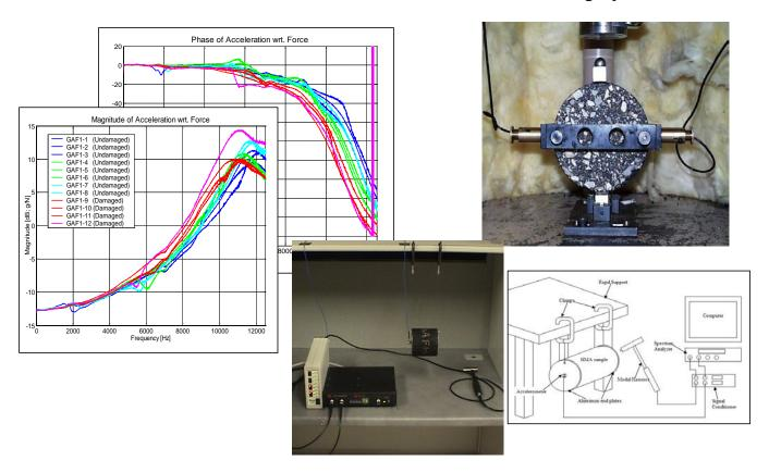
Modal impact testing and acoustic performance testing is used for the determination of material suitability for a variety of applications. Comparative signatures are used for application suitability and material acceptability
