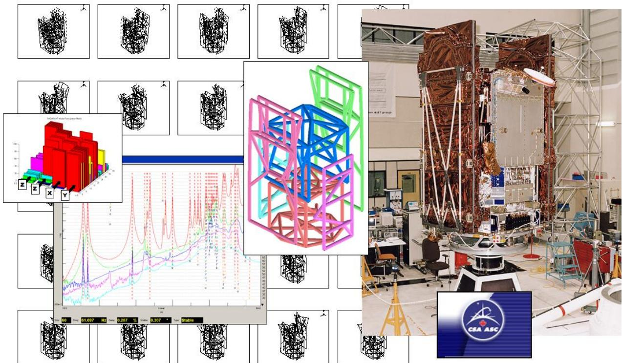
Modal testing of large spacecraft structures requires multiple input multiple output excitation techniques. High modal density requires accurate testing techniques and modal parameter estimation techniques to acquire data suitable for correlation to detailed analytical models.
