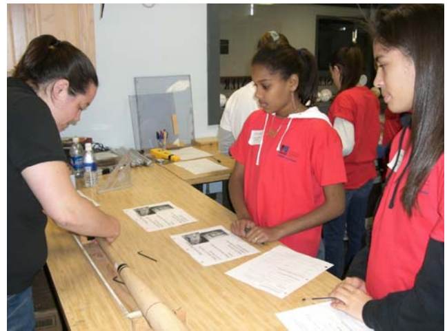
Sarah Tremblay of the Baseball Lab and TEAMS students determine the center of gravity of a baseball bat.
