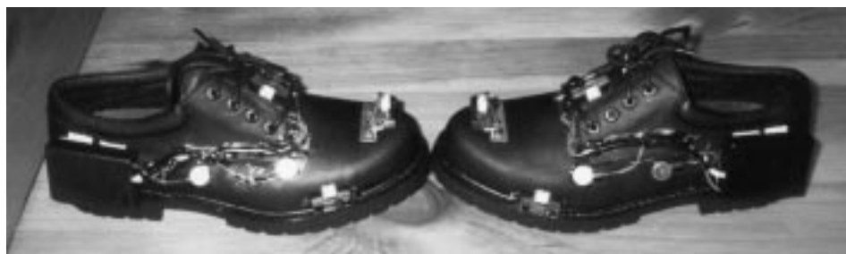
▲ Three sensors on each shoe (on the toe, the laces, and the side) locate obstacles in the front, above and to the side. The person is alerted by three vibrating motors connected to the sensors. The system is controlled by a AAA battery pack that contains three batteries and all the circuitry.
