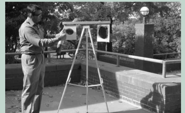
▲ Richard Lemoine, assistant director of Environmental Health and Safety at UMass Lowell, demonstrates how a piece of cardboard treated with PyroTarp paint will not burn through, even when a torch is directed at it. The piece of cardboard on the right was not treated with the fire-retardant paint and burned all the way through during the demonstration, which was presented for a camera crew from FOX 25 News in Boston. The paint is made by Lowell-based Bradford Industries.
