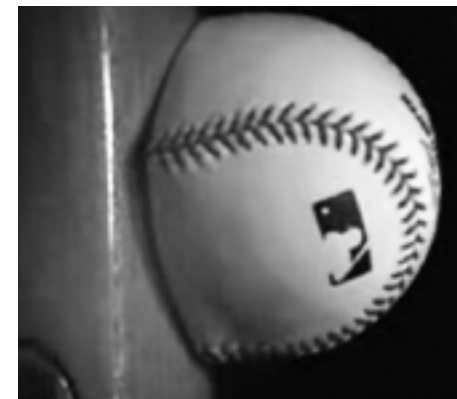
▲ This frame from the YouTube video shows how a baseball gets deformed upon contact with a bat.
